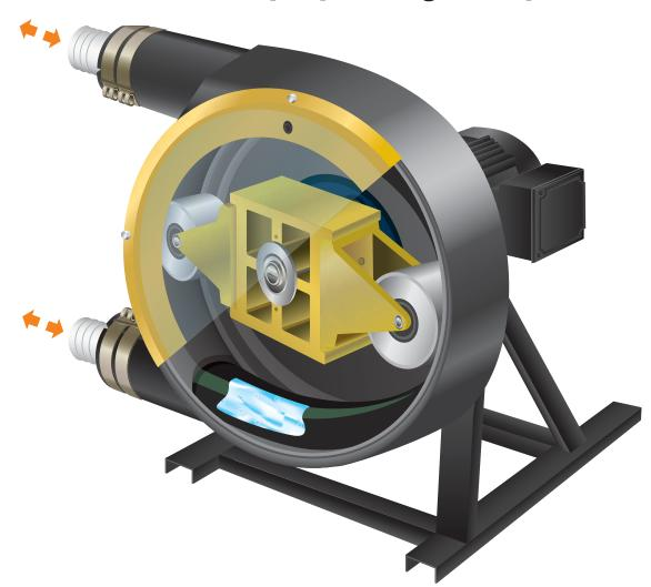
Peristaltic pumps work by compressing and relaxing a hose positioned between a rotating device and a circular pump housing. Vector 2000 Series pumps use rotating rollers that provide the same "push" with far less hose wear.
