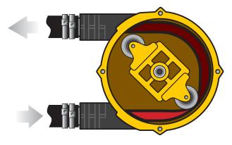
Fluid positioned ahead of the rollers gets pushed forward as the rollers rotate inside of the case.
