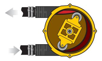
The vacuum draws fluid into the pumping hose, which is then pushed forward by the rollers.
