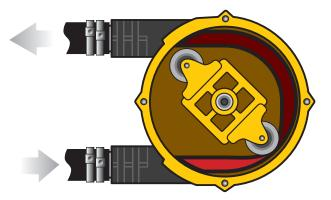
Fluid positioned ahead of the rollers gets pushed forward as the rollers rotate inside of the case.
