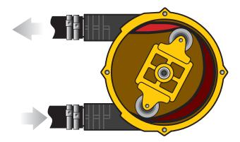
The vacuum draws fluid into the pumping hose, which is then pushed forward by the rollers.
