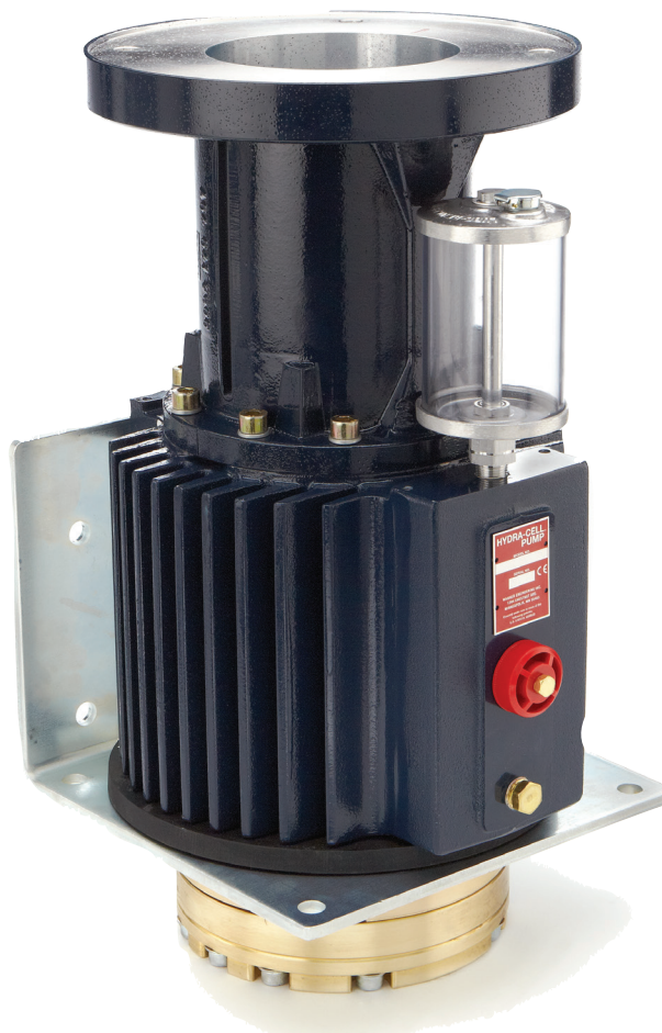
D17 for vertical mounting (including motor adapter, base plate and oil reservoir) shown with Brass pump head.
