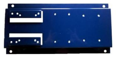
Mount either the pump or the motor to the baseplate, choose whichever has the highest shaft height. In most cases that will mean mounting the motor first.
