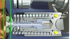
As the diaphragm rolls backward liquid is drawn into the pump chamber and as it moves forward it is discharged through the outlet check valve. The diaphragm movement is minimal, but at a high frequency which translates into very smooth delivery with accuracies exceeding API 675 metering pump standards. There is no dynamic seal, the pump can operate dry if needed and its only limitation compared to progressive cavity pumps are its check valves in terms of viscosity and entrained particle
