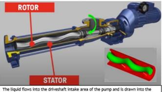
The inguid traws into the driveshaft intake area of the pump and is drawn into the progressive chambers created between the rotor and stator as the rotor rotates. In addition to the interface of the rotor/stator the other wear components include the dynamic seals (mechanical seal and packing) between the drive shaft and gearbox. The maximum particle size is equivalent to the height of the pump chamber.
