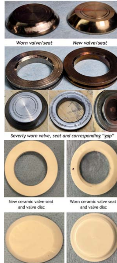
Relative Hardness of Check Valve Materials
