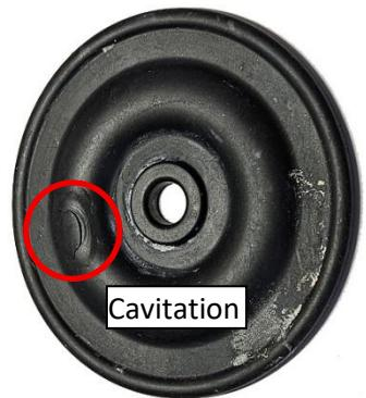
cavitation damage. Prior to 2003 and for some models that were not upgraded until >2004 it was possible to immediately damage a diaphragm via cavitation. The issue at hand was that the resulting vacuum within the pump chamber allowed the hydraulically actuated diaphragm to "over-fill" with oil resulting in mechanical interaction with the outlet check valve leaving a crescent shaped cut along the diaphragm convolute.
